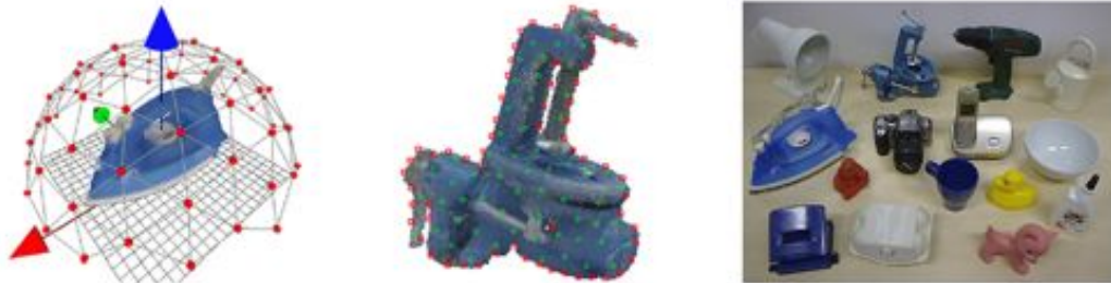
Figure 16: Template generation and the feature points. Left: Red vertices represent the virtual camera centers used to generate templates. Middle: The color gradient features are displayed in red and surface normal features in green. Right: 15 different texture-less 3D objects used. (Courtesy of [Hinterstoisser et al., 2012])
